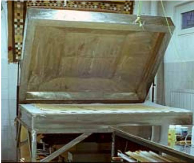
Fig. 4. The steam chamber
