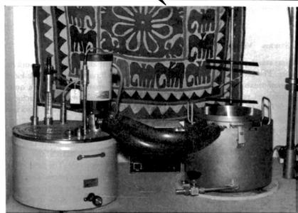
Fig. 7. Paste stirring vessel.
