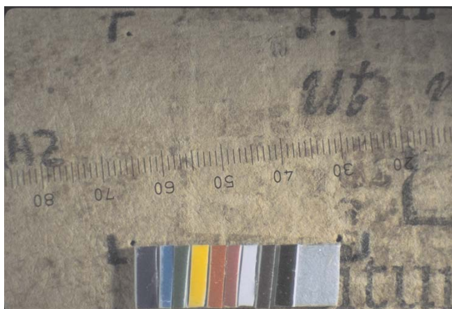
FIGURE 5 Laser cleaning with \lambda = 532 nm of superficial deposits of adhesive glues. a Rubber-based adhesive, F = 0.8 \text{ J cm}^{-2} , N = 2 ; b mixed starch- and protein-based adhesive, F = 0.4 \text{ J cm}^{-2} , N = 2
